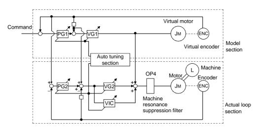
The block diagram of the Servo Amplifier servo control section is shown above. (The current loop is omitted.)
